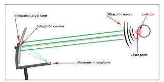
By focusing the ultrasonic waves in the parabolic mirror, even the smallest leaks of 0.8 l/min (approx. € 8 p.a.) can be located with pinpoint precision (± 15 cm) at a distance of up to 10 to 15 m.
